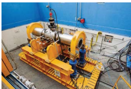
Bending test (12" 900# ball valve for subsea application).
