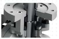
3 Downstream non-floating seat ring is shouldered into the body. The seat-to-ball contact is fully lapped metal-to-metal, eliminating particle entrapment.
